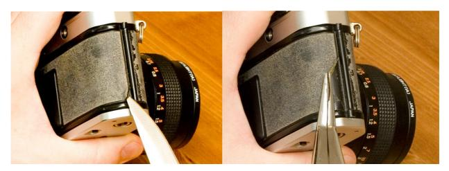
Using alcohol and a Q-Tip (Cotton Bud) and old cloth, please remove all of the old adhesive. It is very important to remove all traces of the old adhesive. If any of the old adhesive is left on the camera, the new adhesive will not stick to it. You may need to clean the camera two or three times with the cloth and alcohol.
